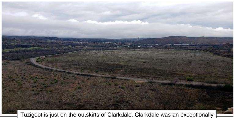
large producer of copper. The entire field below is tailings from the copper mines. When the orange dust storms became too much to handle, the ore company covered them up and revegetated them.
