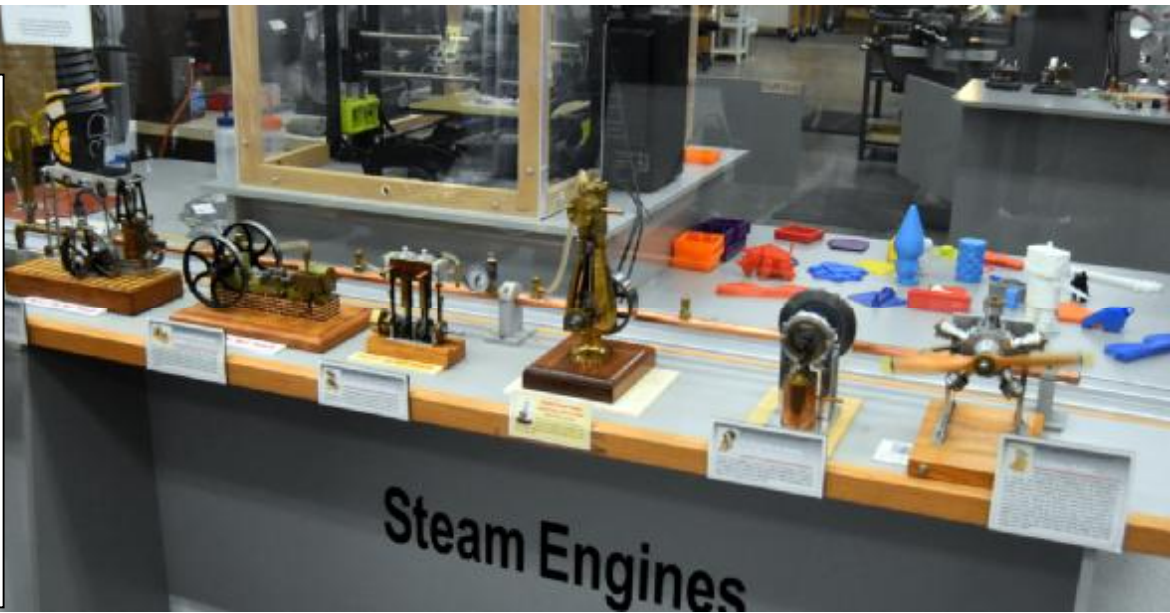
The copper pipe along the back supplies steam to these engines. You can't tell in a photo, but they are all running. Then an engineer gave a little demonstration of how things are made, without a computer.
