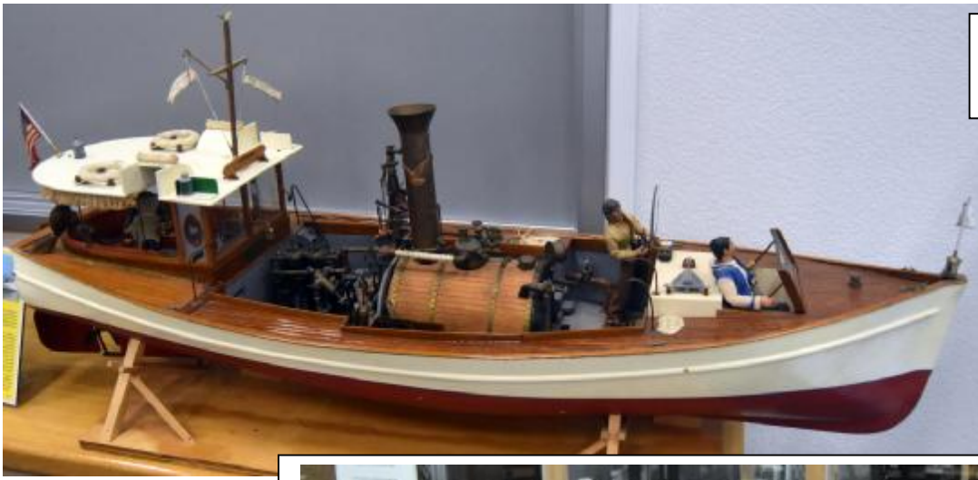
The copper pipe along the back supplies steam to these engines. You can't tell in a photo, but they are all running. Then an engineer gave a little demonstration of how things are made, without a computer.
